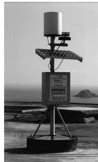
Figure 2. The automatic raingauge.
